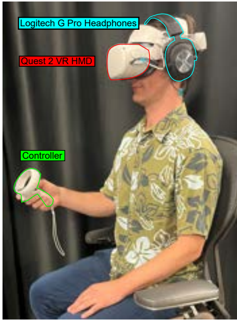
Fig. 1. Annotated photo showing a participant completing the experiment, wearing a Meta Quest 2 HMD and Logitech G Pro VR Headphones, while holding the controller in their dominant hand.
