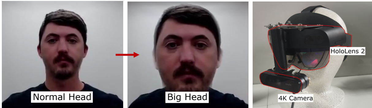
Figure 1: Illustration of real-time magnification of heads in augmented reality (AR). From left to right we see a normal head, “Big Head” or magnified head, and an annotated photo showing our AR prototype with a 4K camera mounted on a HoloLens 2.
