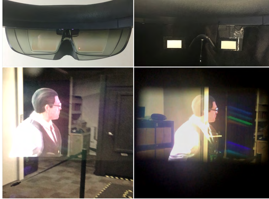
Figure 5.4: View conditions and captured photos for each condition: (left) unrestricted, (right) restricted. The augmented field of view is 30^{\circ} \times 17^{\circ} . The images here show only a small peripheral area because of photographing constraints. The peripheral FOV perceived through the HoloLens is much larger.
