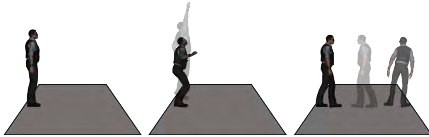
Figure 5.3: Obstacle behavior from left to right: (standing) the human stands and looks around idly, (jumping) the human jumps in place around 22 times/min, and (walking) the human walks back and forth along the shorter edge of the platform at .27 m/s.
