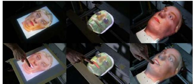
Figure 1: Touch sensing on one flat and two head-shaped rear-projection surfaces. Detected touches prompt graphical responses.
