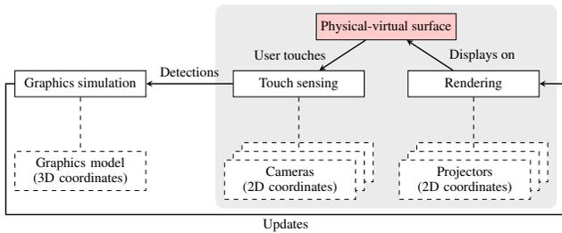
Figure 3: Overview of touch sensing method. Touches on the surface are imaged by cameras and converted to 3D graphics model coordinates to trigger appropriate updates.
