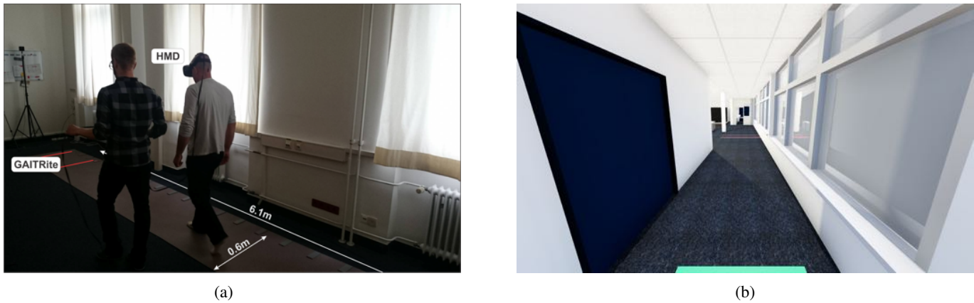
Fig. 1: Experiment setup: (a) A participant walks in the real workspace with an HMD over the GAITRite walking surface, and (b) participant's view on the HMD.
