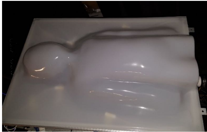
Figure 3.12: Vacuum formed acrylic shell
