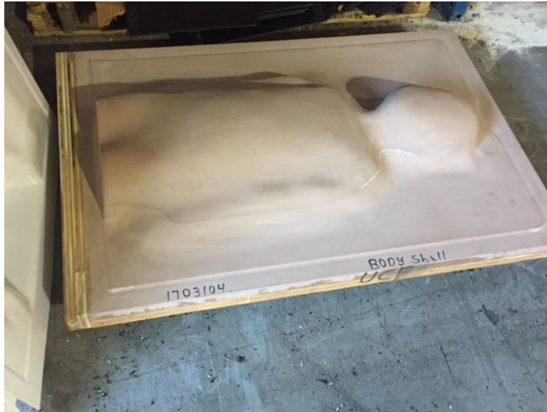
Figure 3.11: Mold milled using the 3D design
