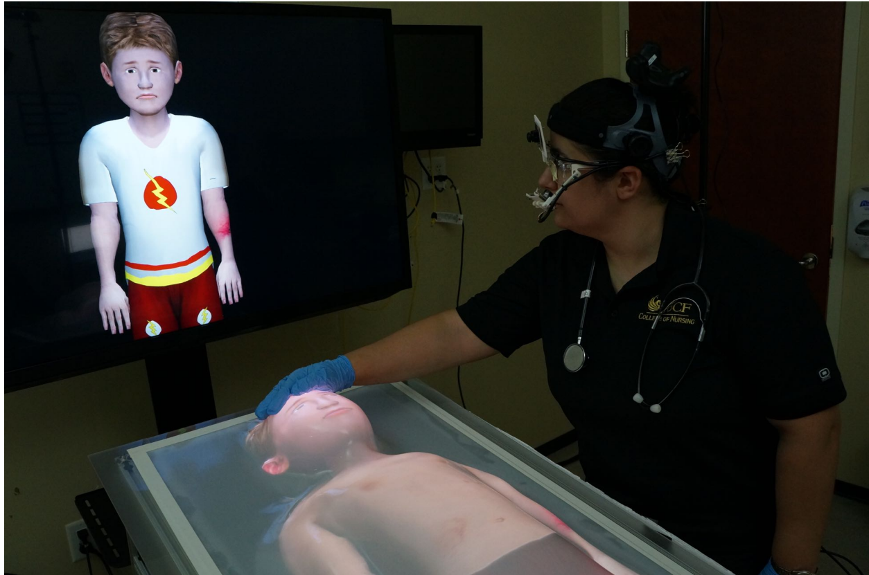
Figure 5.1: A human subject examining a virtual child in a medical pediatrics training scenario associated with a controlled study. The face of the user, who is wearing eye-tracking gear, is blurred to hide their identity. Here, the physical-virtual patient simulator comprises separate dynamic visuals on a TV screen (left), with heat and pulse sensations integrated into a three-dimensional mannequin-like shell with static visuals (below). In this condition the shape is matched—the shell is the same shape as the embodied virtual agent (a child), and yet the imagery is not matched—the dynamic visuals of the child are separated from the child-shaped shell.
