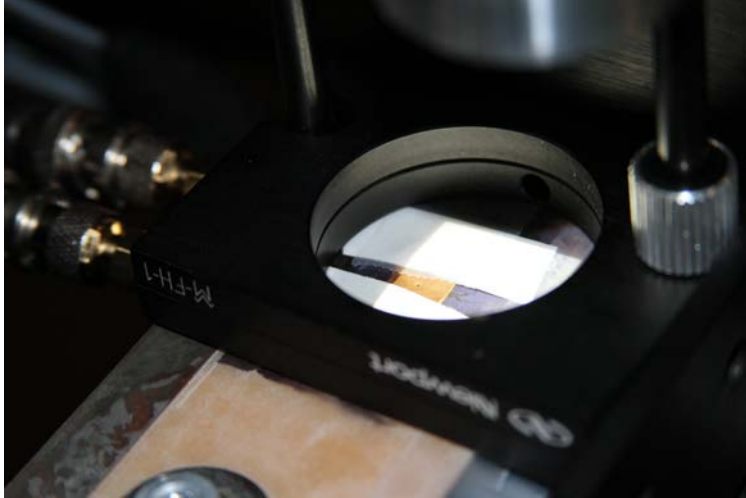
Figure 3.10: Light measurement sensor and barrier. The light-to-voltage sensor is located behind the pinhole (approximately 0.25 mm in width), visible in the copper segment between the two strips of white tape inside the circle. This circle has a diameter of 3.8 cm.
