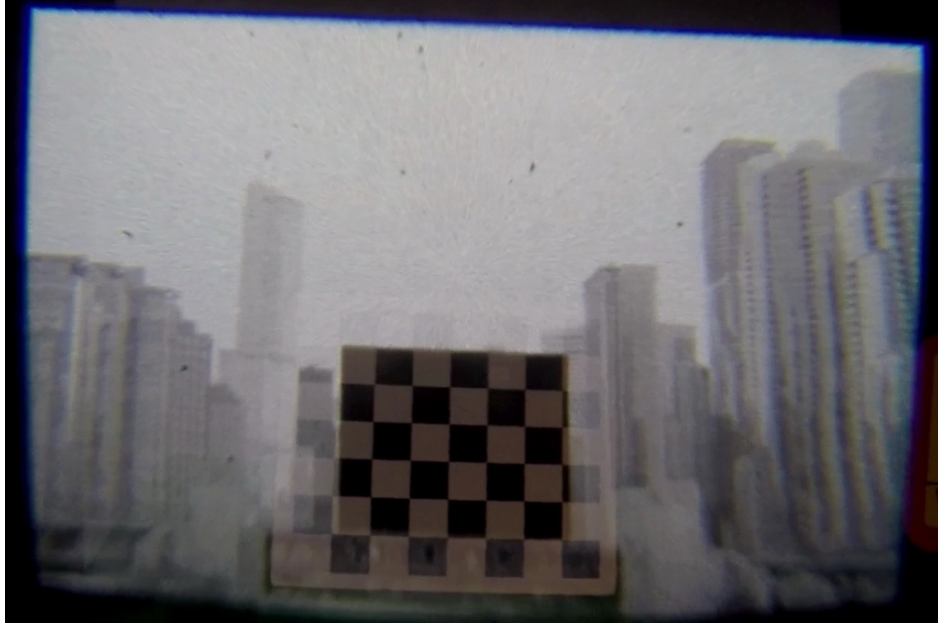
Figure 4.3: A sample frame using our latency compensation algorithm under fast panning motion (50 °/s) where the majority of the field of view is dominated by a off-kilter grayscale planar image of a city skyline, in which a small cutout region is registered to the physical checkerboard. Note that the cutout and the checkerboard interior are well aligned and details in the city photo are visible.
