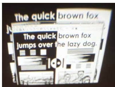
Figure 4.2: Output imagery for tests with the EEM scheme where the input imagery varied over time (increasing from left to right). The input consisted of a sequence where the input in Figure 4.1(a) filled the background and a window containing a smaller version of the same image was moved across the screen.
