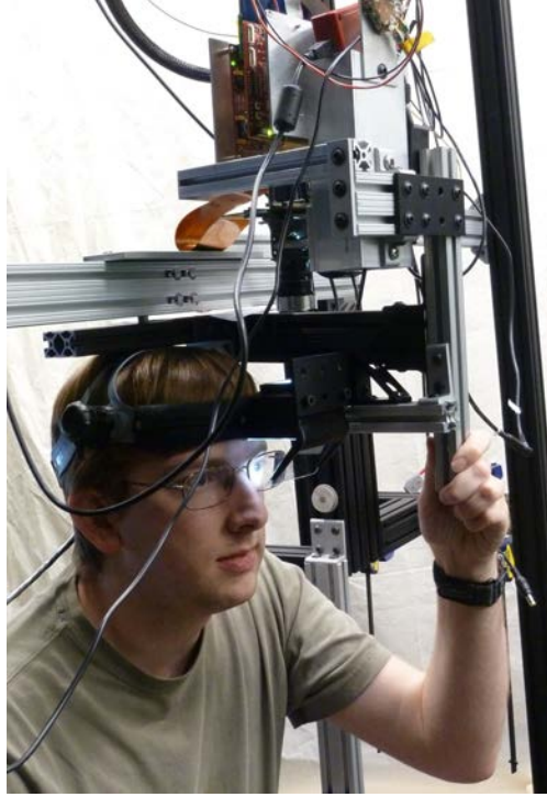
Figure 1.3: A user “wearing” our AR display. The monocular virtual imagery is presented to the user’s left eye.
