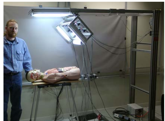
Fig. 6. Retained camera setup for 3D Medical Consultation prototype. Left: simulation. Below: acquisition rig.
