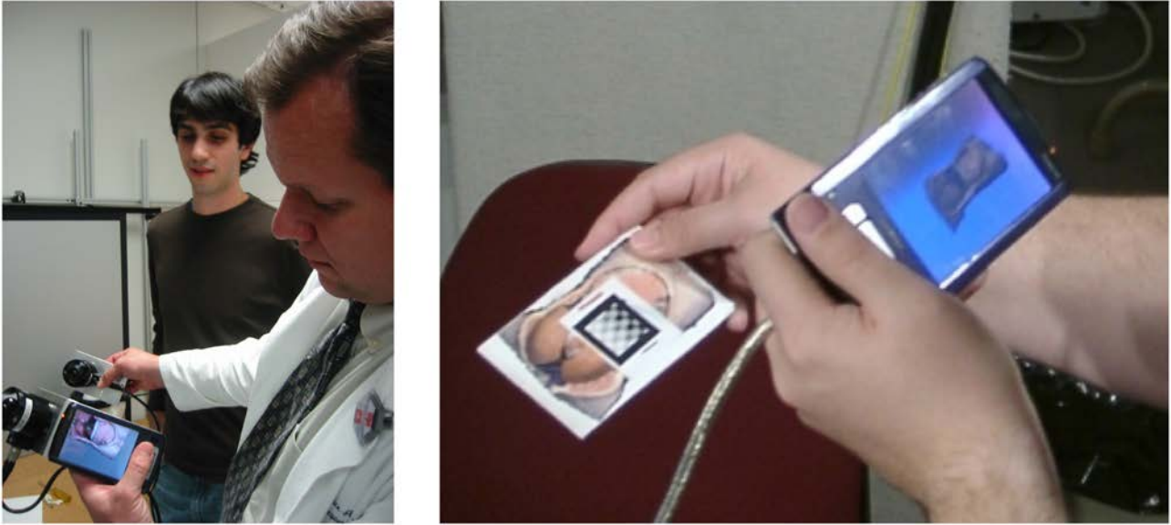
Figure 6: Left: Our first tracked PDA prototype used a HiBall-3000 TM tracking system [2], with sensors mounted on the PDA (Toshiba e800, left hand) and the surrogate (right hand). Right: Our current prototype uses a PointGrey DragonFly camera [1] mounted on the PDA (left hand). The prop (right hand) has a printed image of our training torso on it, along with a grayscale pattern. We use the ARToolkit [8] to track the surrogate with respect to the PDA (camera).
