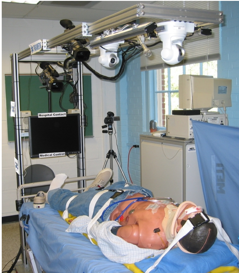
Fig. 6. Human patient simulator staged as an accident victim for the experimental evaluation. Note the 2D video cameras and display mounted on the overhanging structure.
