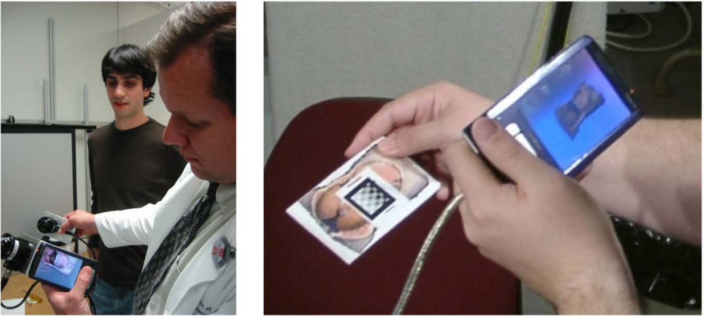
Fig. 5. Left: Our first tracked PDA prototype used a HiBall-3000 TM tracking system [16], with sensors mounted on the PDA (Toshiba e800, left hand) and the surrogate (right hand). Right: Our current prototype uses a PointGrey DragonFly camera [17] mounted on the PDA (left hand). The prop (right hand) has a printed image of our training torso on it, along with a grayscale pattern. We use the ARToolkit [18] to track the surrogate with respect to the PDA (camera).
