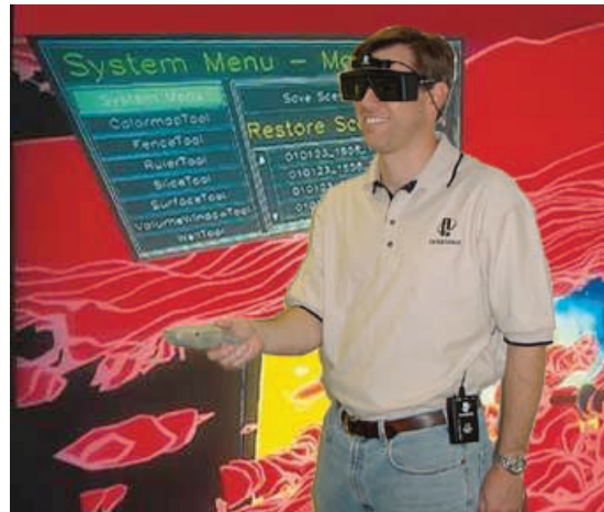
12 InterSense IS-900 wireless tracker option, including a belt-worn battery/radio module for the head tracker. For the wand, the battery and radio are built into the handle.
