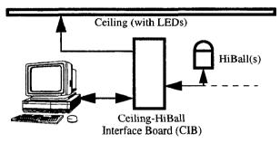
Figure 2. A block diagram of the HiBall tracking system.
