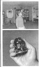
Figure 1. Left: the original UNC optoelectronic ceiling tracker in use, and a close-up of the head-mounted display and sensor fixture, along with the signal processing and communications electronics pack. Right: the new system in use, and a close-up of the self-contained HiBall with lenses and part of the cover removed. See also the color plate Welch 1.
