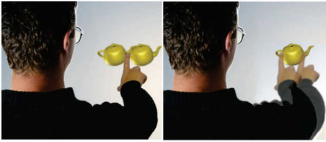
Figure 1. Illustration of the main problem for touch interaction with stereoscopic data. The user is either focused on the finger, which makes the selection ambiguous, or on the object, which disturbs the visual perception of the finger.
