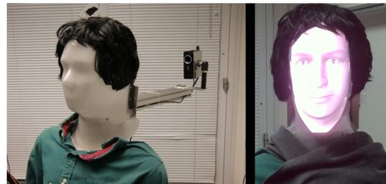
Figure 1: At left, the physical-virtual avatar (PVA) apparatus. At right, the participant’s view of the PVA when in use. The face is animated, computer-generated imagery projected onto the inside of the plastic face. The projector can be seen in the center of Figure 1, Left.
