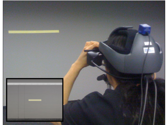
Figure 2: Picture taken during the psychophysical calibration process. A participant at a fixed position compares the size of the horizontal stripe in the real world with the virtual stripe displayed on the HMD (see inset).
