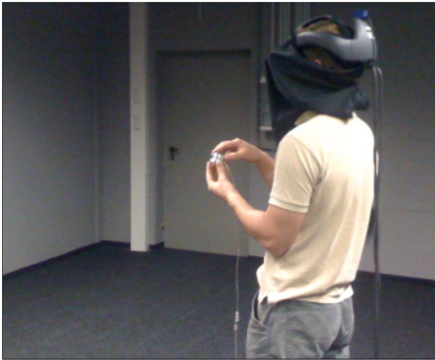
Figure 4: Photo from the experiment showing a subject with the ProView SR80 HMD adjusting the GFOV with the PowerMate.
