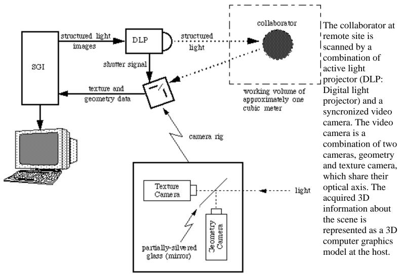
The underlying difficult correspondence problem from stereopsis is often reduced by projecting structured light patterns. We currently use binary coded vertical bars. A camera looks at a set of patterns to distinguish between all the projected vertical bars. To distinguish between 512 projected columns 9 patterns are required.
