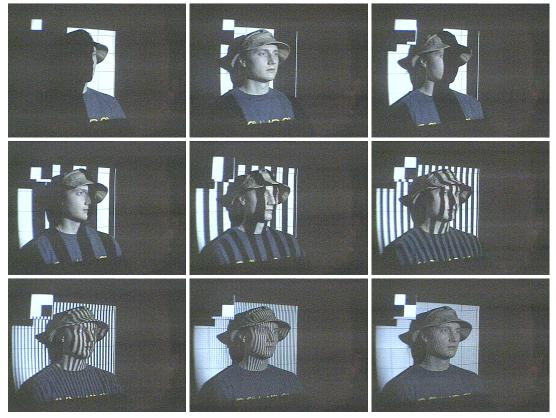
We hope to make the projected patterns imperceptible to human eye. Binary image of the pattern and its inverse are projected in quick succession. This appears as a uniform grey level. A camera synchronized to the projector however can detect the pattern by capturing only the first half duration.
