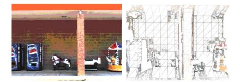
Figure 15: Left: Input image. Right: Illustration of multi-resolution triangular mesh
