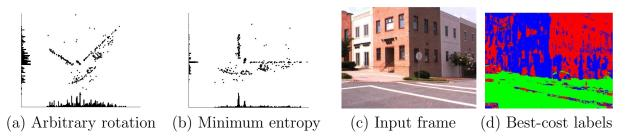
Figure 6: Minimum entropy optimization. The 3D points are projected in the direction of gravity. Then they are rotated into the basis formed by u and v and histograms are generated. The histograms of (a) have more entropy than those of (b). (b) corresponds to the correct surface normals. (c) image from original viewpoint. (d) Best cost selection (ground points are labeled green, and facade points are labeled red or blue).
