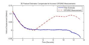
Figure 4: Above: Errant vertical motion measured by the INS/GPS and the Kalman filter estimated vertical motion.
