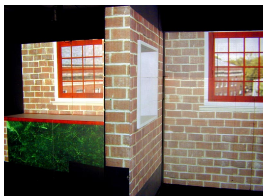
Figure 1. We use Styrofoam blocks to construct a geometrically simplified replica of the scene. The Styrofoam blocks are used as display surfaces on which view-dependent imagery of the scene is projected. Most of the geometric complexities in the scene, such as the window frames, windowsills, the pass-through in the middle wall, and the molding around it, are left out in the simplified replica. (This figure is reproduced in color on page 200.)
