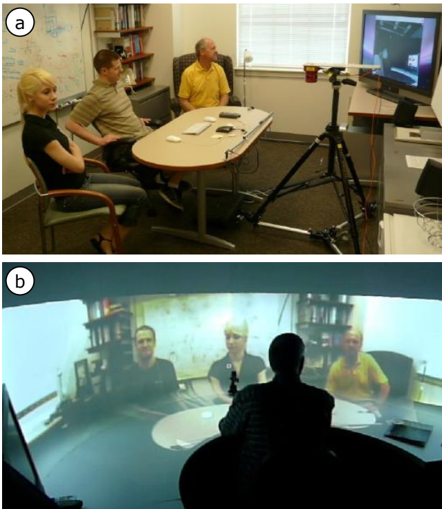
Figure 8: Mock-up of remote panoramic video for avatar control. A PointGrey Ladybug camera is used to capture panoramic imagery of a remote scene in (a). The real-time panoramic video is mapped to a projector-based 270° surround display as shown in (b). The Ladybug would eventually be mounted above the SLA.
