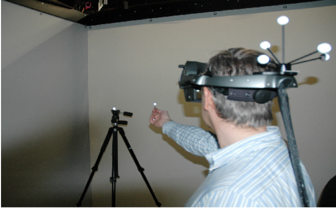
Fig. 1. A user aims at a stationary and a hand-held marker. Positions of 3-DOF markers and 6-DOF HMD-attached marker are tracked by infrared cameras.
