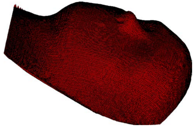
Figure 3. The resulting structured coded light scan for the physical–virtual patient head after interpolating to 70511 vertices.
