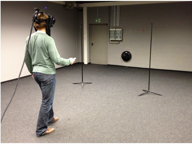
Figure 5: Experiment setup: subject walking in the direction of a target displayed at eye height for a distance indicated by the center of two vertical poles.
