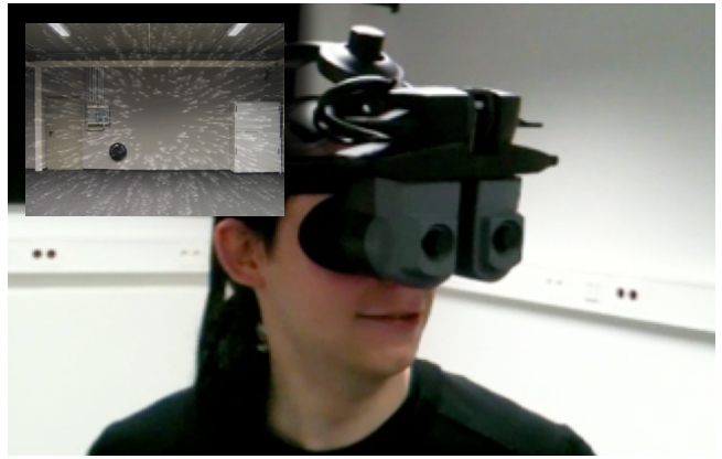
Figure 1: Photo of a user wearing a tracked NVIS nVisor MH-60V video see-through HMD. The inset shows an illustration of the resulting expansive optic flow field during forward movements.
