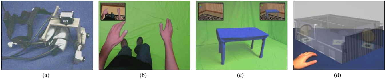
Figure 1: Virtual studio: (a) modified video-see-through eMagin Z800 head-mounted display, and (b) augmented virtual self-representation (inset showing augmented virtual view), (c) augmented virtual desktop workspace (left inset showing applied green and blue color key segmentation, right inset showing applied green color segmentation only), and (d) markers used to place and combine designs.
