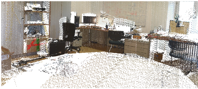
Figure 2: Views of a user walking towards a table in the Automation Lab PCVE (ca. 3.4 \cdot 10^6 points in 62 scans rendered at about 250 fps).
