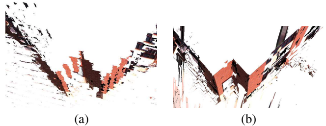
Figure 4. Stereo depth maps rendered as 3D models. (a) Fronto-parallel sweep only. (b) Multiple sweeping directions.
