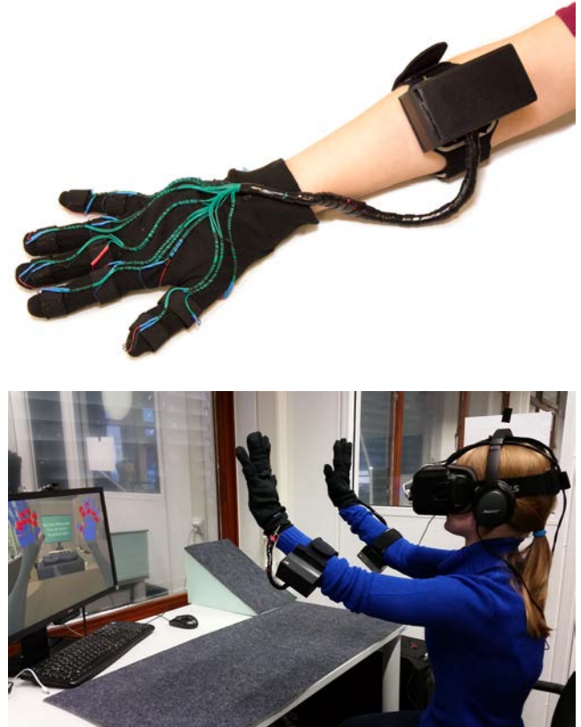
Figure 2: Images of (top) self-made glove with the electronic case attached to the forearm, and (bottom) participant interacting with the VR application, wearing the pair of gloves and the Oculus Rift DK2 with the Leap Motion attached in front to facilitate the hand tracking.
